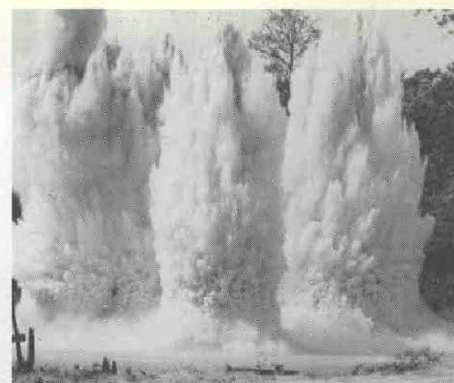
Fig. 3. MINES, under 1½ to 7½ feet of water, were exploded by FAE munitions that actuate when warhead probe fuze impacts water surface, exploding center warhead burster and dispersing FAE cloud above water; cloud detonation transmits explosive shock into water to detonate mines.
