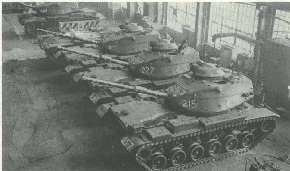
M60A1s waiting to be taken to the one-mile oval test track adjacent to the Detroit Arsenal Tank Plant where a final 50-mile test is conducted before shipment to combat elements.
