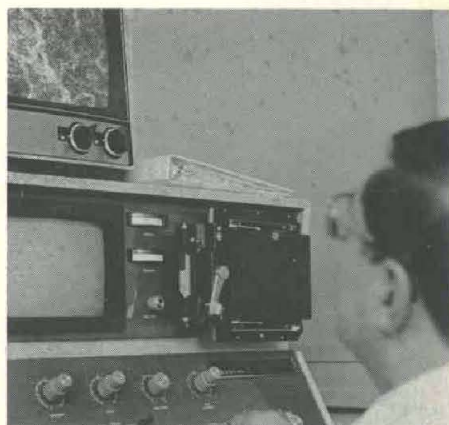
METALLURGIST observes surface characteristics of a part of a vehicle steering column magnified 1,000 times by using a new Electron Scanning Microscope at APG.
