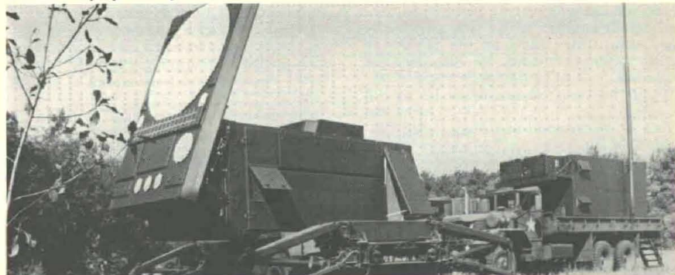
MOBILITY OF THE PATRIOT missile system was demonstrated recently when it was driven out of the Raytheon plant at Bedford, MA, mounted on an SM-860 trailer towed by an M818 tractor and set up in minutes in a wooded field by soldiers from HQ U.S. Army Mobility Equipment R&D Command, Fort Belvoir, VA. It was the first emplacement demonstration of the U.S. Army's new air-defense system. At the left is the radar and right the engagement control section. Equipment will be sent to White Sands (NM) Missile Range for testing this year.
