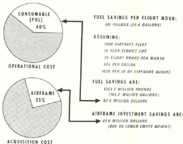
Fig. 2. Effect of Engine Technology on Aircraft
