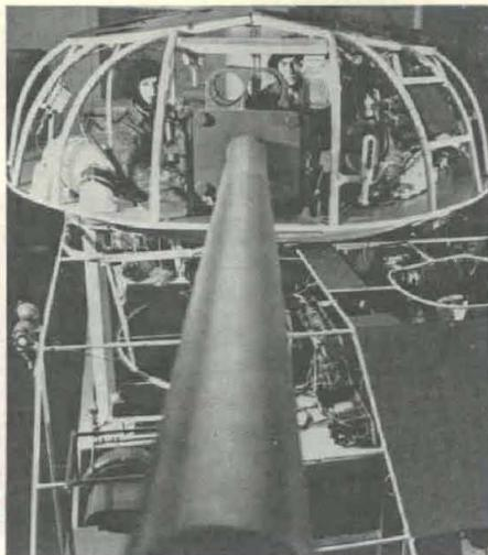
Fig. 5. Cutaway Simulator of T-55 Tank.
