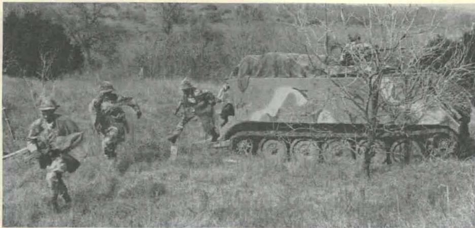
CAMOUFLAGE PATTERNS designed by the U.S. Army Mobility Equipment R&D Command have replaced the olive drab and white star on all major tactical items. The designs disrupt the signature characteristics of vehicles; reduce contrasts with soil and vegetation, and distort internal shadow areas.
