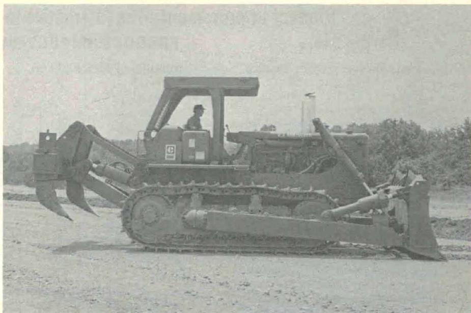
D8K diesel tractor with bulldozer and ripper.
