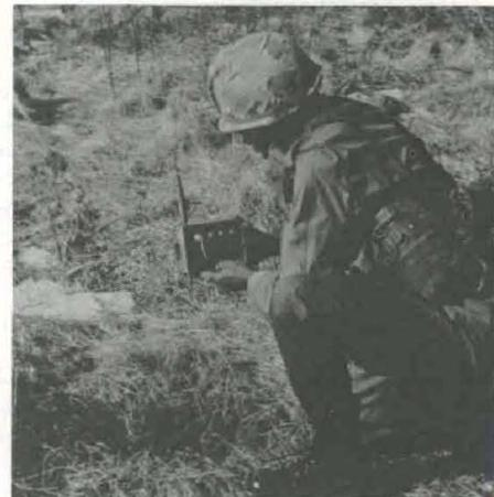
TYPICAL HAND-EMPLACED sensor, with all codes set, is planted in a hole where it will be covered by grass and leaves, leaving only the antenna exposed.
