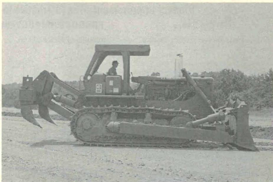
D8K diesel tractor with bulldozer and ripper.
