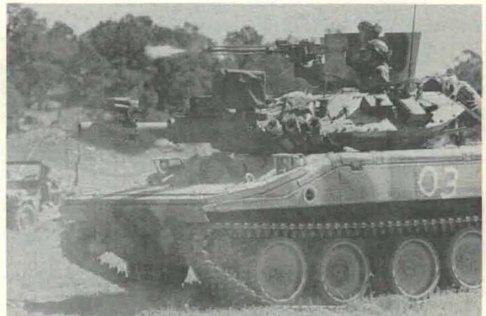
M551 Sheridan equipped with MILES training system. The main gun has the capability of firing one of three lasers to simulate the Shillelagh missile, 152 main gun and coaxial machinegun. Additionally, the cupola-mounted 50-caliber machinegun has its own laser transmitter capability.
