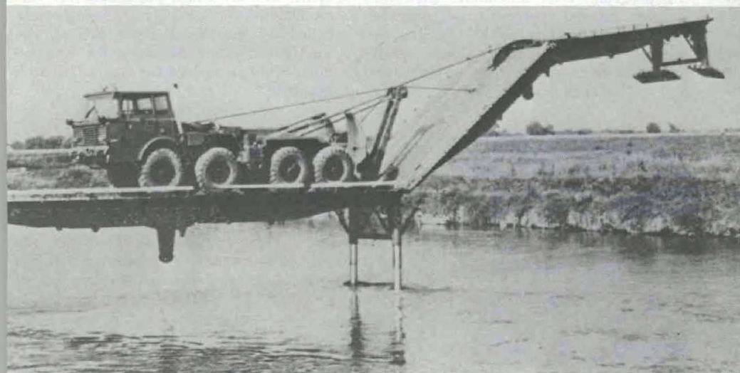
Czechoslovakian AM-50 truck-mounted bridge.
