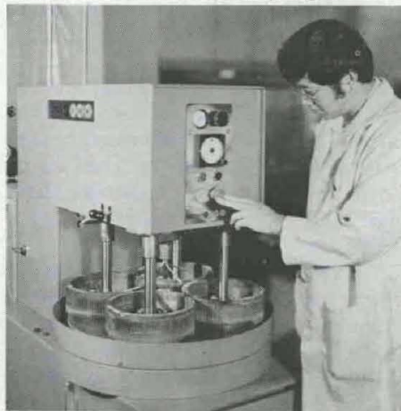
FREE ABRASIVE GRINDING MACHINE enables an operator to prepare concrete to a smooth flat surface that can be examined with a stereoscopic microscope to determine air content of the specimen at Waterways Experiment Station.
