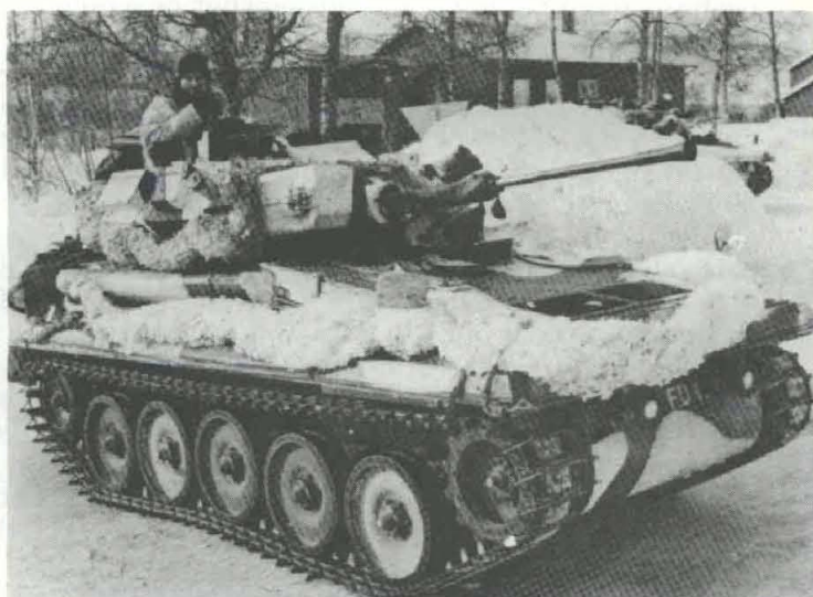
British Scimitar, CVR(T), mounting 30mm Rarden gun (1973).
