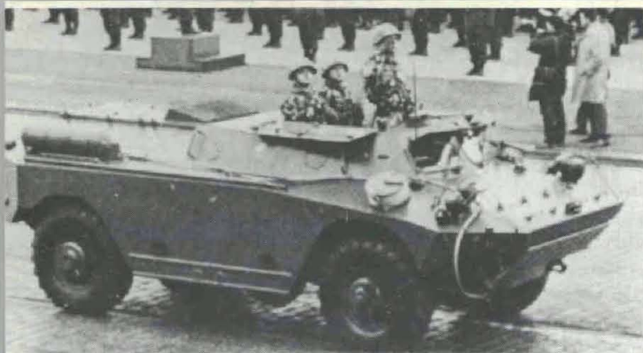
Czech OT-65, 4x4, scout vehicle, produced in Hungary (1963).
