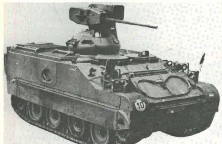
Royal Netherlands Army M113A1 Command and Reconnaissance Carrier rearmed with Oerlikon KBA-B, 25mm automatic cannon (1966/1978).
