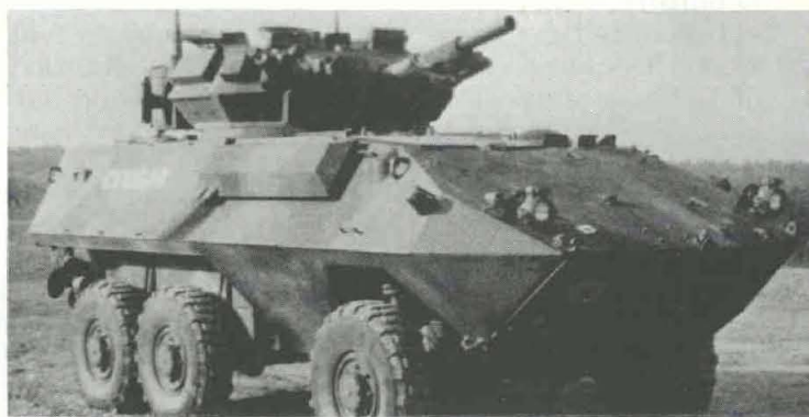
Canadian Cougar, Fire Support Vehicle mates Scorpion turret with Swiss MOWAG Piranha, 6x6, APC chassis.
