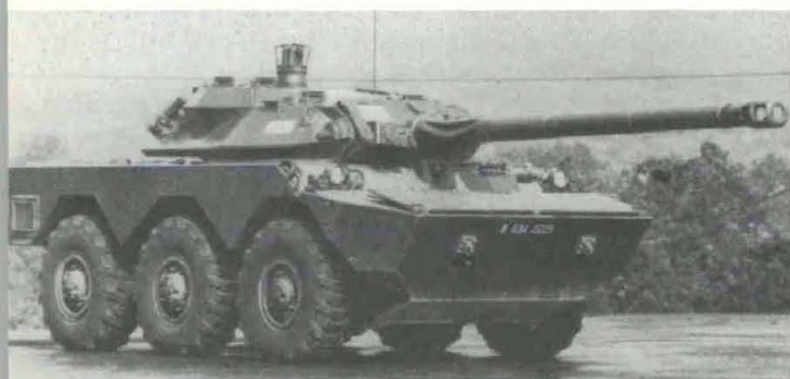
French AMX-10RC, 6x6, equipped with 105mm gun and advanced fire control, designed for corps-level reconnaissance and as a heavy-fire support vehicle by mechanized infantry divisions (1979).
