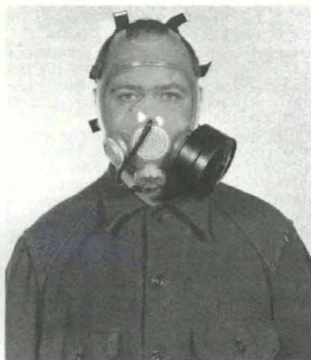
XM30 PROTECTIVE MASK is being developed jointly by the U.S., which is developing the face piece, and Canada developing the canister. The mask features a clear face piece that allows greater visibility than current masks and, if adopted, will replace the M17A1, M24, M25A1 and M9A1 masks.
