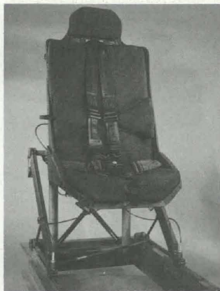
Fig. 2. Boron Carbide/Kevlar Seat for Black Hawk
