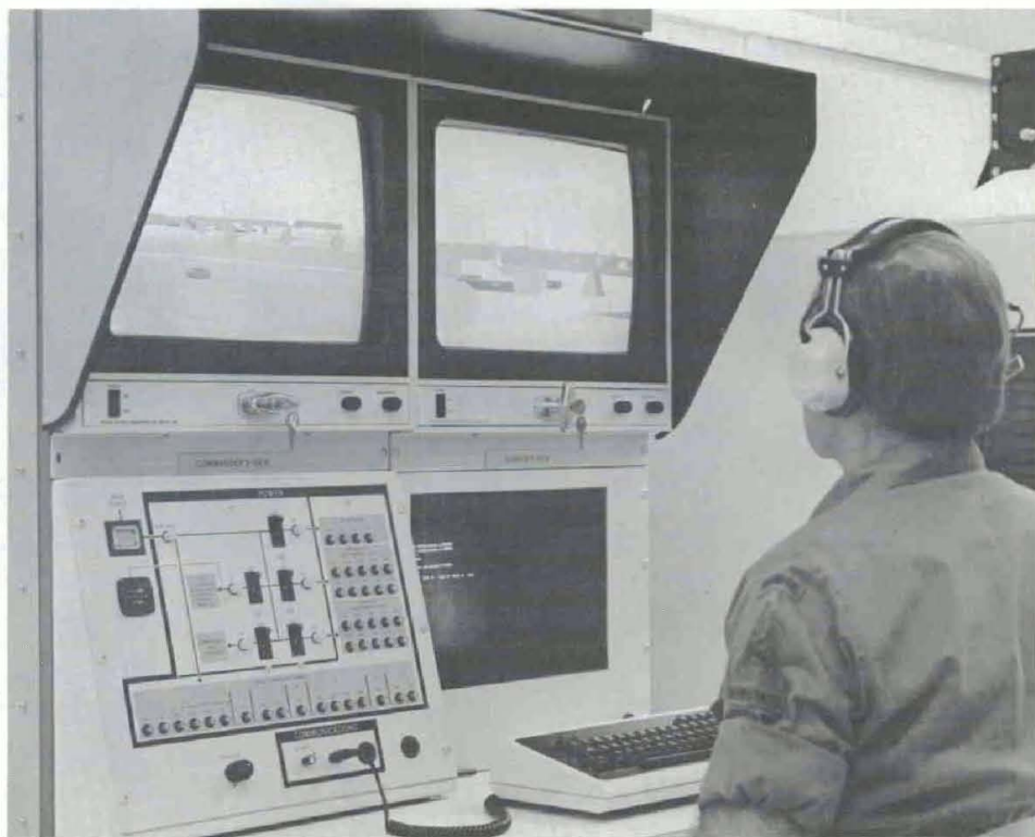
Fig. 2. COFT Instructor/Operator Station Showing Video Displays
