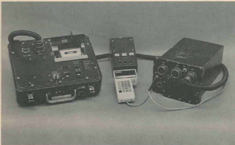
COMPONENTS of Vehicle Monitoring System: From left — Data Retrieval Unit; Maintenance Action Indicator, with Set Communicator in foreground; and the Vehicle Monitoring Systems Electronics Assembly.
