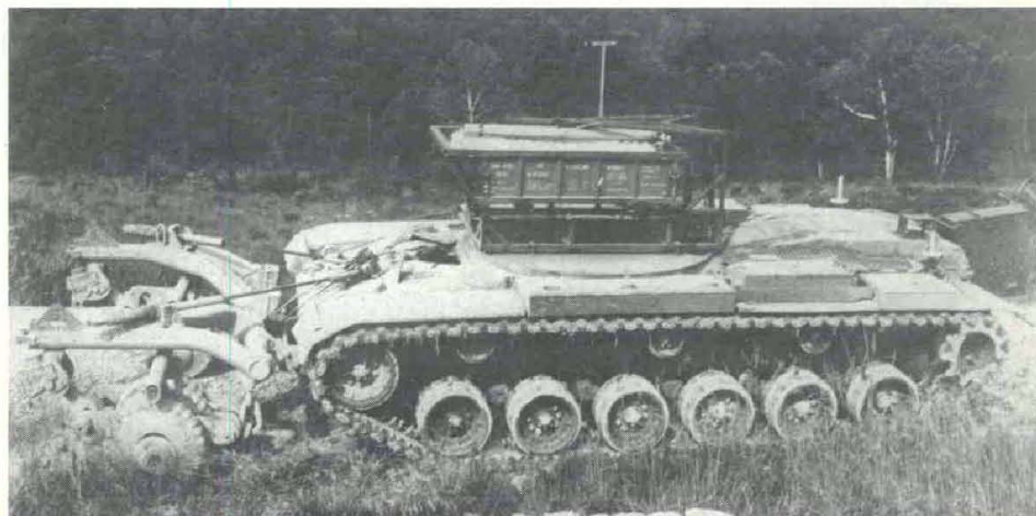
COUNTER-OBSTACLE VEHICLE — Modified M60A2 tank chassis, fitted with a mine-clearing roller, a Marine Corps M58A1 mine-clearing line charge, and a Clear Lane Marking System (CLAMS) that marks safe lanes breached by the system.
