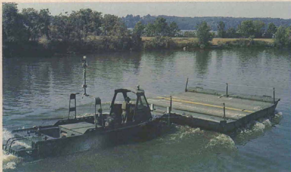
RIBBON BRIDGE ERECTION BOAT moves a bridge bay into position at MERADCOM's ponton basin.
