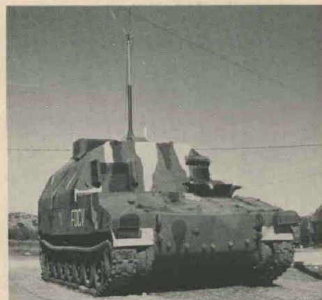
NBC-protected, fire direction center vehicle, designed, fabricated and tested by HEL in 1981, is scheduled for joint-effort testing by HEL and the Chemical Systems Lab.
