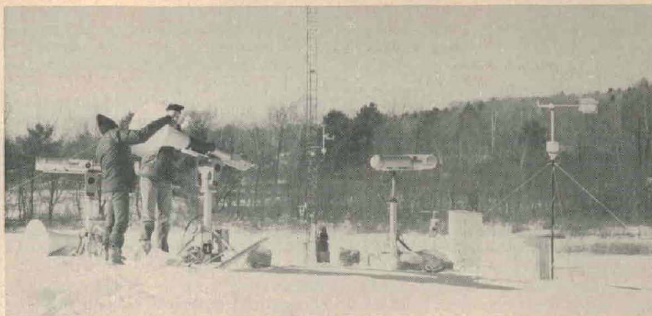
SNOW characterization instrumentation being used by CRREL in SNOW field experiments include (from left) holocamera, electro-optical particle-size probes, and snow-content meters.
