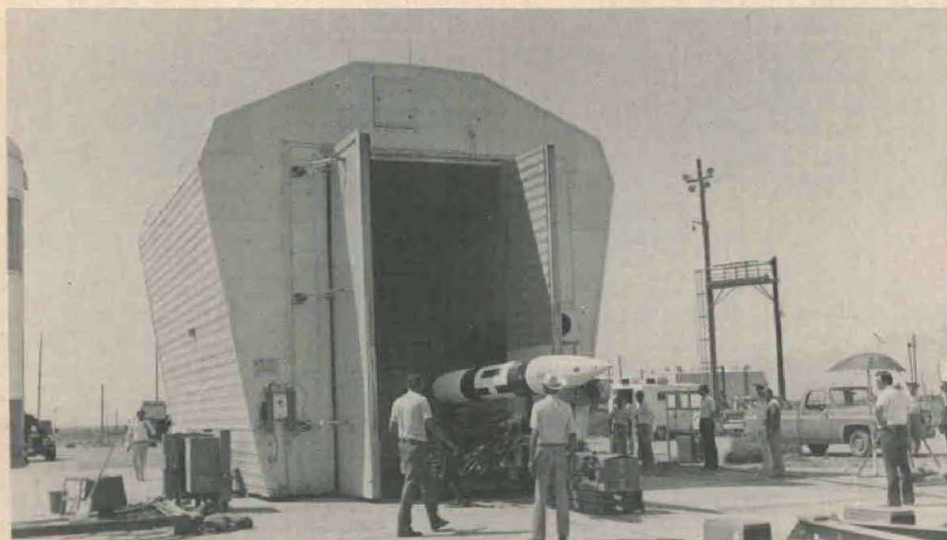
SIG-D (Simplified Inertial Guidance-Demonstration) missile emerges from a climatic chamber prior to launching at White Sands Missile Range (WSMR), NM. The SIG-D test program is being carried out at WSMR by the U.S. Army TECOM, which tests proposed Army materiel at nine installations and activities.
