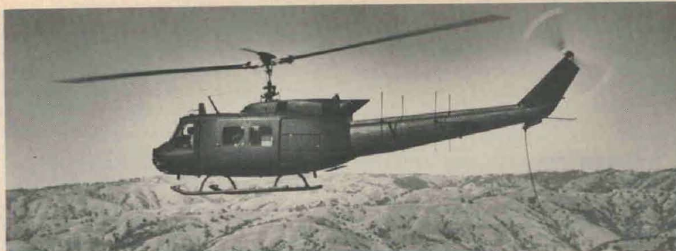
AN/ALQ 151 electronic countermeasure system, developed at the Signals Warfare Laboratory, has intercepting, jamming and direction finding capabilities.
