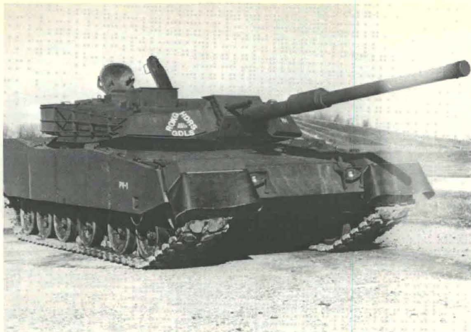
An automotive test rig (ATR) being tested at the Materiel Testing Directorate as the main battle tank for the Republic of Korea shows its kneeling capability made possible by its hydro-pneumatic suspension system. A second prototype, a fire control test rig, is also undergoing tests at MTD.
