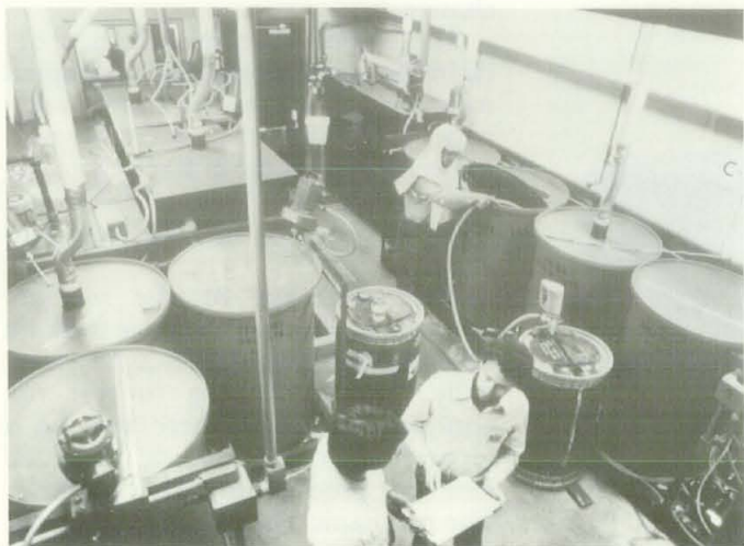
Workers at the Tobyhanna plant begin the purification process by separating contaminants from waste water pumped into the facility from metal finishing operations.
