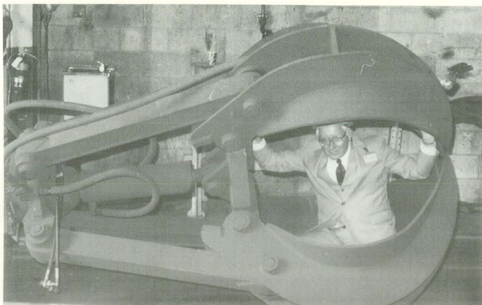
Weapons System Manager Richard R. Rogowski inside grapple attachment for telescopic arms. The grapple is one of two special arm attachments for the test bed, and has a capacity of 2½ tons.
