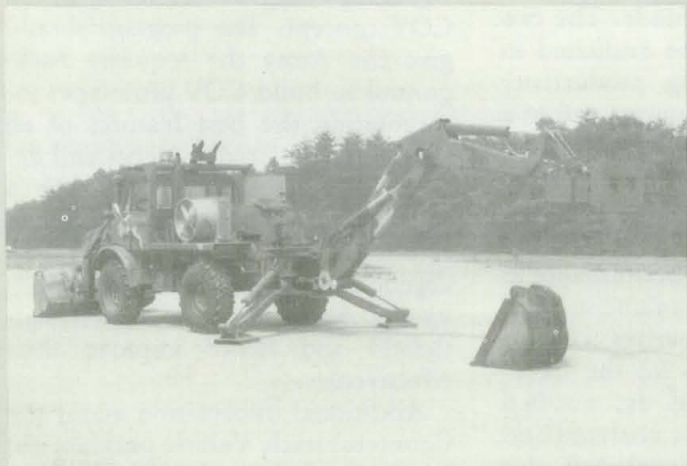
The specially adapted cross-country vehicle equipped with microprocessor-controlled backhoe and manipulator arm will enable an operator to load and unload ammunition from inside the cab of his vehicle.
