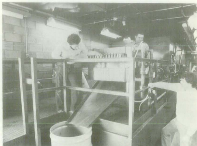
When the treatment process is completed, sludge is drained off the disposal.
