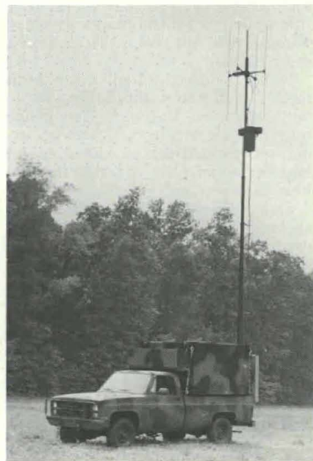
The AN/TRQ-32 (V-1) mounted on a 1 1/4-ton truck.
