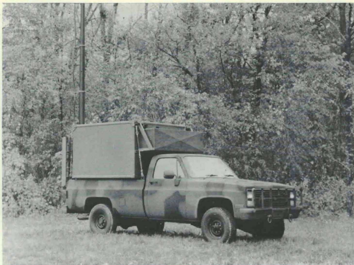
The Commercial Utility Cargo Vehicle (CUCV) with a AN/TRQ-32 signal warfare shelter.
