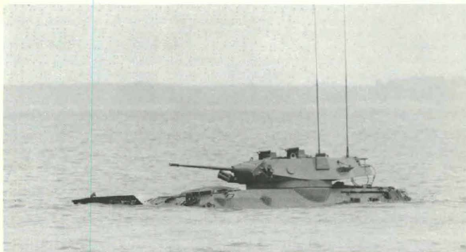
A light armored vehicle (LAV)25 demonstrates its amphibious capability while undergoing testing in a water area of the Proving Ground.
