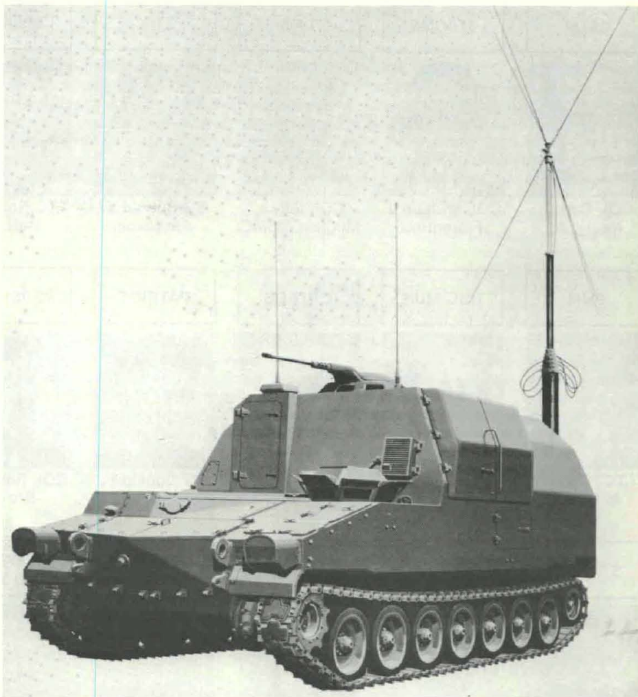
The Army Human Engineering Lab's command post vehicle is part of a test bed program that will enable data to be collected on command, control, and communications operations in nuclear and chemical environments.
