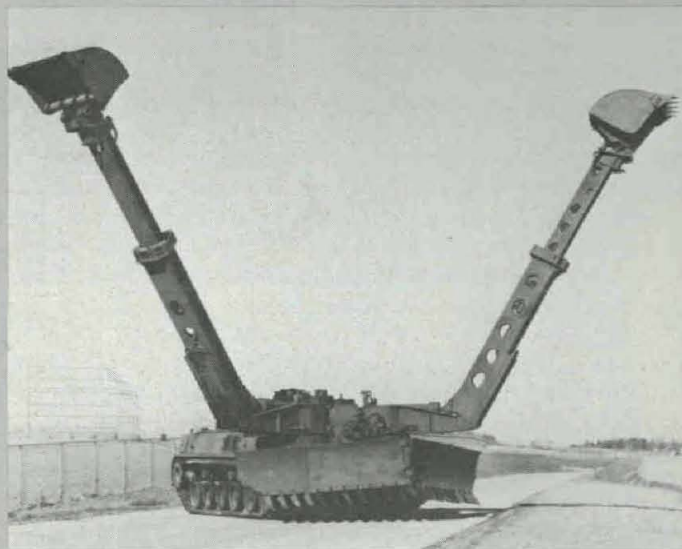
Counterobstacle vehicle experimental prototype with full-width mine plow/bulldozer and telescoping arms mounter with excavators.
