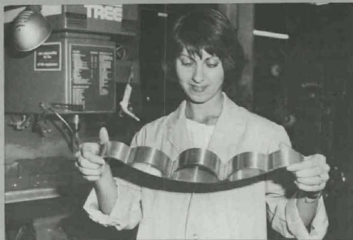
Catherine Kominos examines a completed model of her new bridge design. If tests are successful, this concept could reduce the weight of Army bridges by almost 20 percent.
