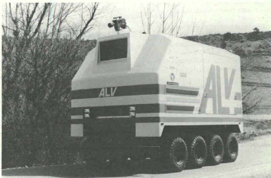
The DARPA autonomous land vehicle (ALV) demonstrator developed for early road following and cross-country testing.
