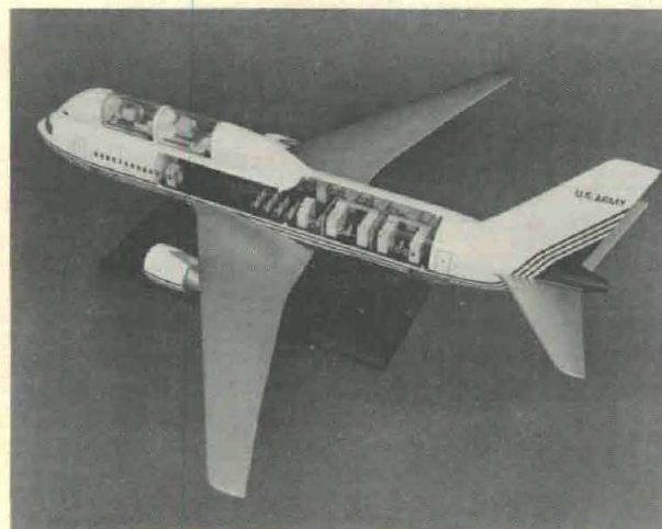
This model is a preliminary concept of how a commercial jet will be modified in the Airborne Optical Adjunct (AOA) project. The upper fuselage will house two sophisticated optical sensors. Experimental flights of the AOA will examine how airborne optical sensors can be used to augment ground-based BMD radars.
