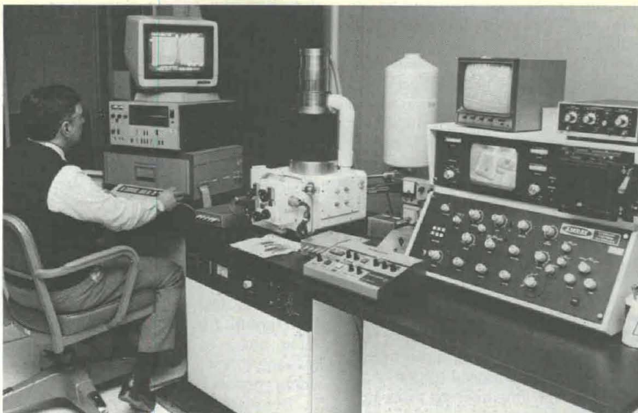
Scanning electronic microscope with Energy Dispersive X-Ray Analysis and Image Processing System used by Electronics Technology and Devices Lab for electron beam diagnostics and failure analysis of microelectronic devices.
