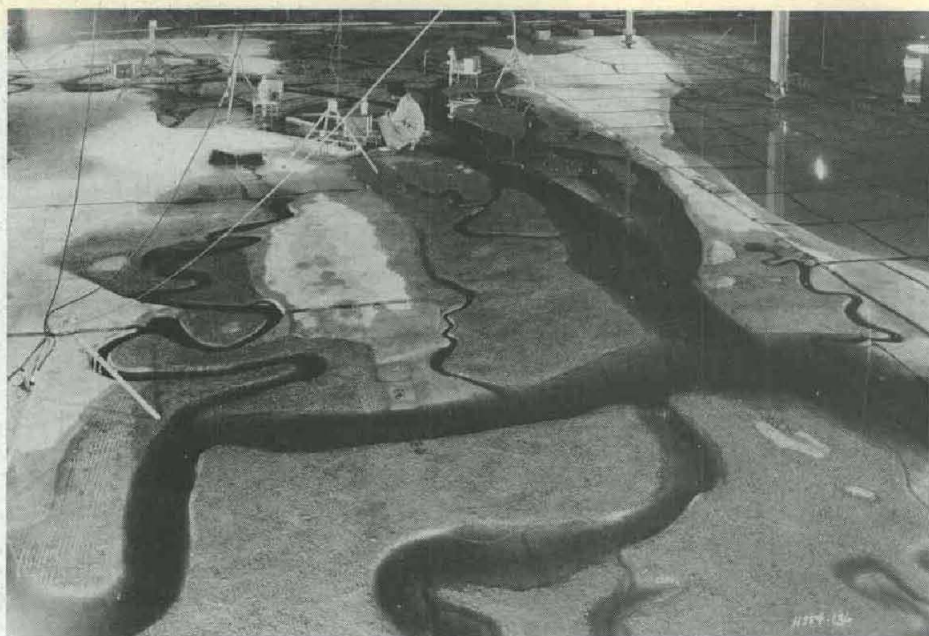
WES physical model of the Trident submarine base at Kings Bay, GA.
