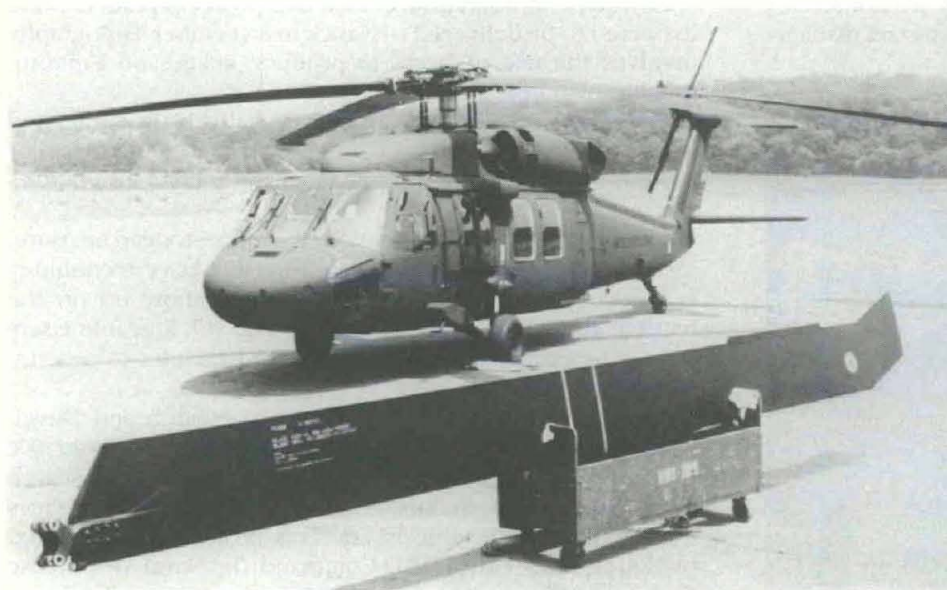
Low cost composite blade for the UH-60 Black Hawk.
