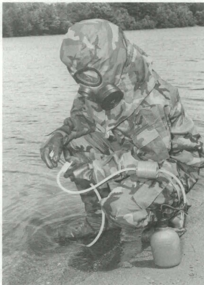
Hand pump and filtering cartridge for purifying water.
