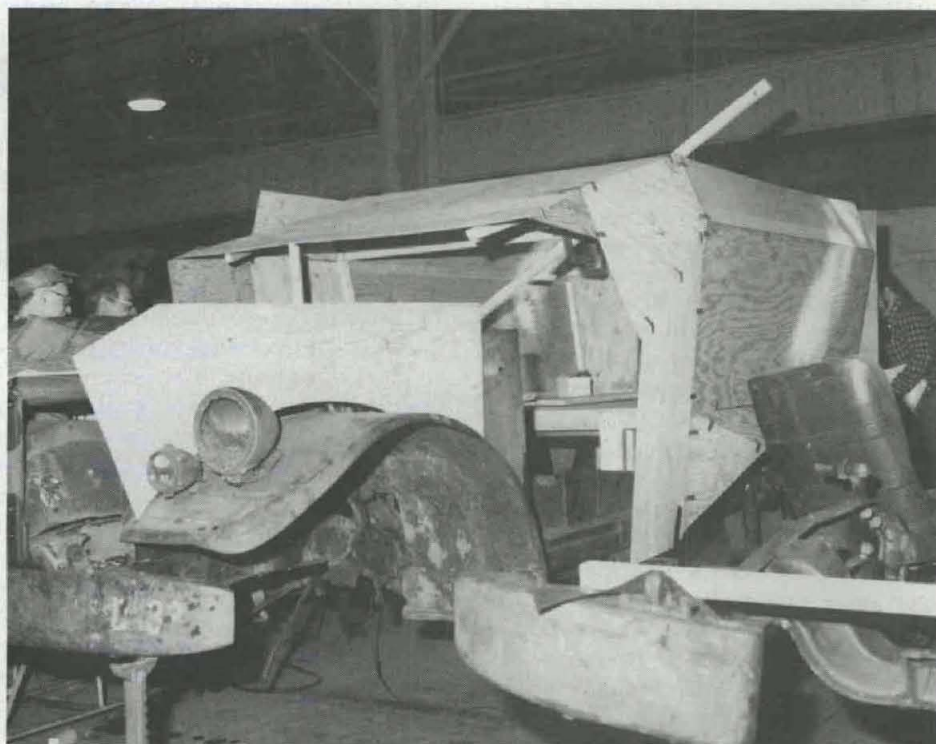
Prior to building the prototype from armor, a wooden mock-up was made to validate the design.
