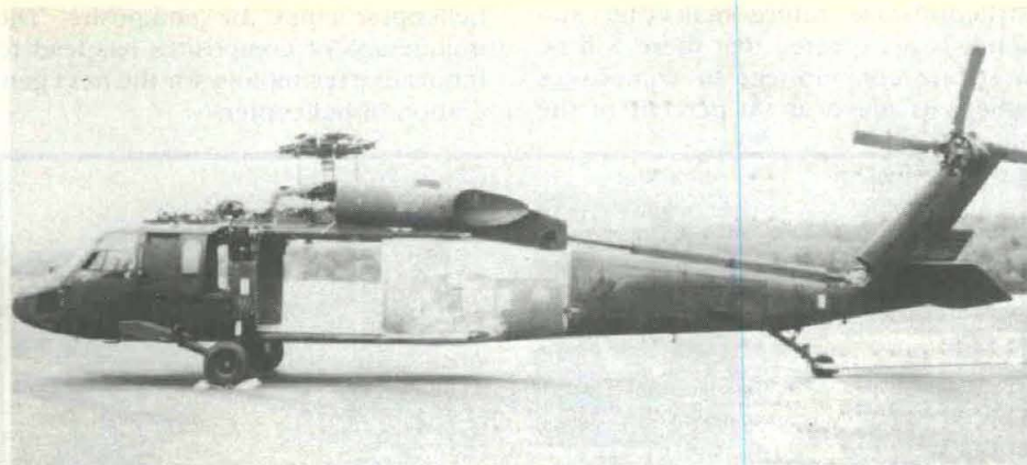
Composite rear fuselage for the UH-60 Black Hawk.
