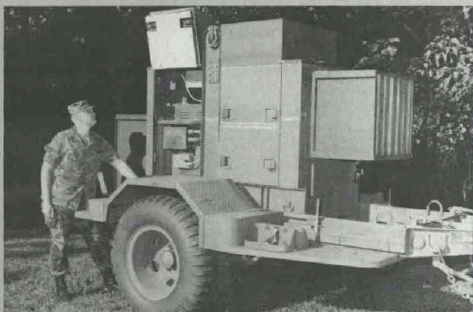
Generator which was modified to meet noise ordinances in populated areas is now about as loud as a normal conversation. Modifications were made by the Belvoir RDE Center to permit its use with the Army's Regency Communications Network.
