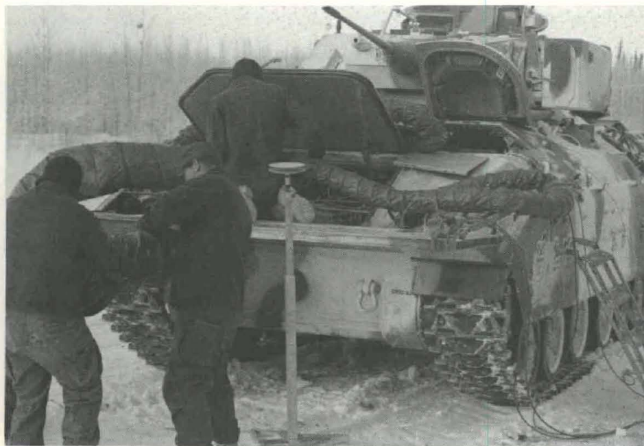
M2 Bradley Infantry Fighting Vehicle being prepared for cold-start testing at CRTC.
