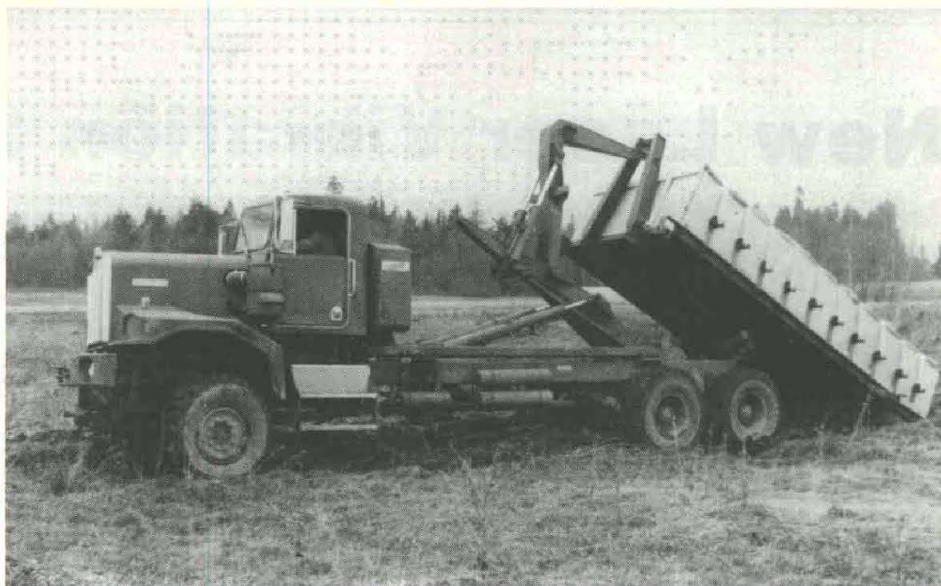
Cargo truck with hydraulic pickup unit in a downloading mode.
