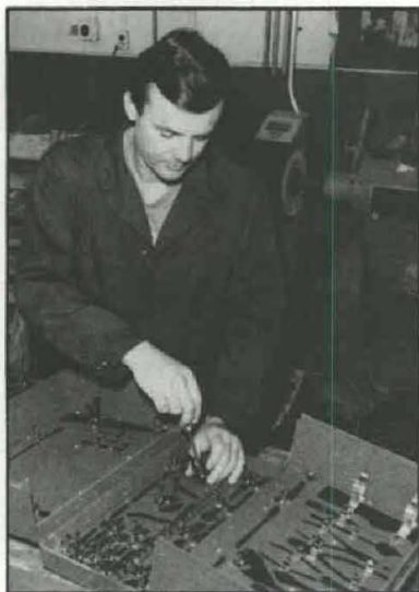
James Skates, model maker, installs a retaining clip in the New Aircraft Tool System.
