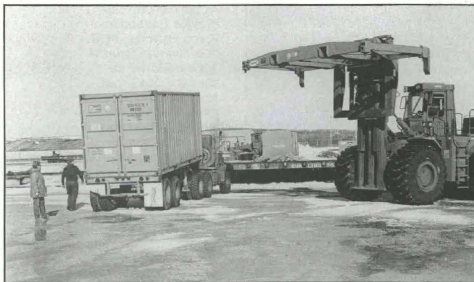
Preparations are made for container handling/loading for a rail impact transportability test. The container handler is approaching the commercial container for removal from the chassis and placement on a railcar.
