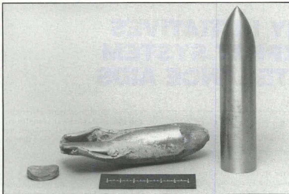
Figure 2. A "new" projectile next to a post-test or "used" projectile
