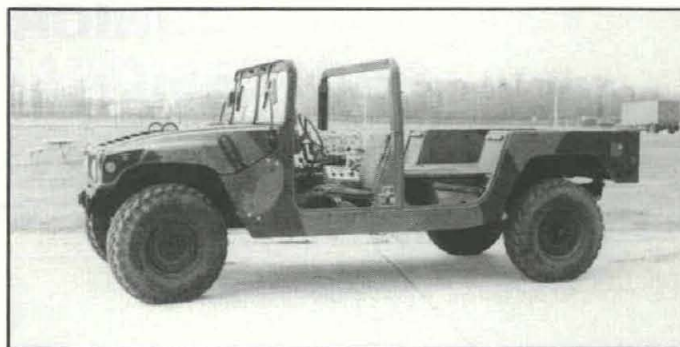
This modified HMMWV has a control system that lets an operator drive it and do tasks from a remote-control station.
