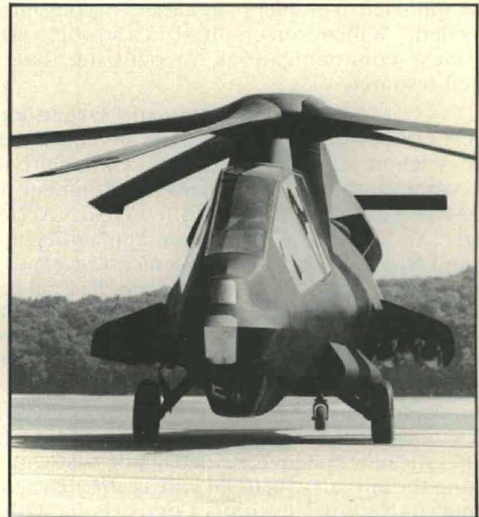
Head-on view of Boeing Sikorsky Light Helicopter First Team's full-scale mockup shows Aided Target Detection/Acquisition pod on nose, 20-mm Gatling gun cannon, retractable missile bays, five-bladed rotor.
