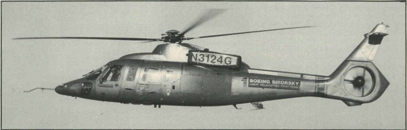
Boeing Sikorsky Light Helicopter First Team FANTAIL demonstrator aircraft is shown during flight testing at Sikorsky's facility at West Palm Beach, FL. Aircraft is a Sikorsky H-76 modified with a FANTAIL antitorque system similar to the one designed for the First Team's Light Helicopter.
