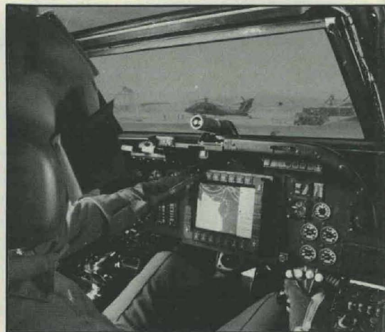
Selected components of the McDonnell Douglas/Bell Helicopter Textron SuperTeam LH mission equipment package have been installed in a prototype Apache helicopter for flight evaluation. The liquid crystal flat panel display is shown in digital configuration.
