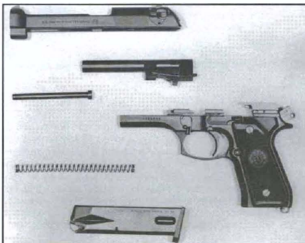
Left Side View of Pistol, M9, Field Strip. The Level of Disassembly of Components (top to bottom): Slide Assembly, Barrel Assembly, Recoil Spring Guide Rod Assembly, Receiver Assembly with Grips, Recoil Spring, and Magazine Assembly.
