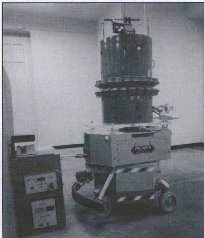
At the end of a tour, an MDARS robot automatically moves to a charging station and plugs itself in.
