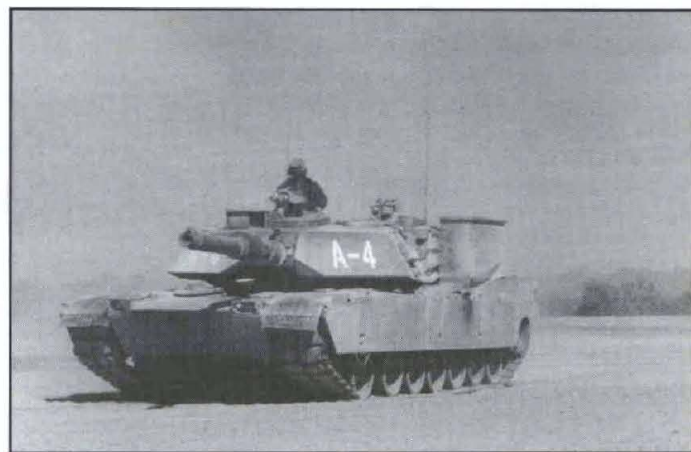
Positioned over the air intake on the left rear sponson of the Abrams, the air induction tower allows clean air to be drawn into the engine.
