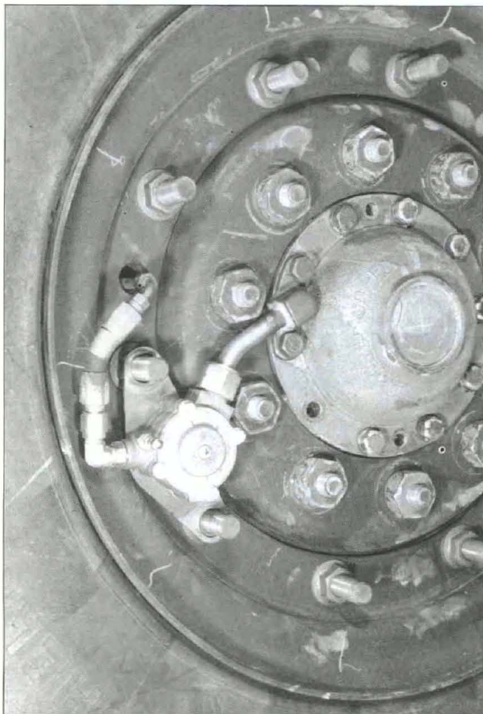
The wheel valve permits air in or out of the tire.
