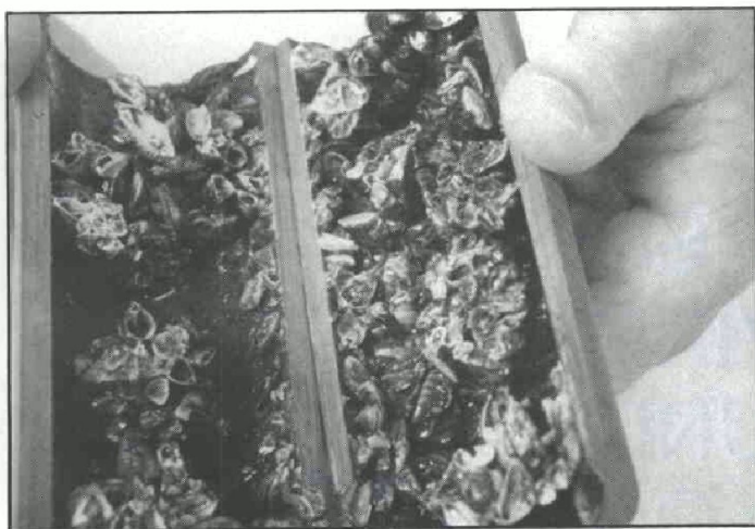
This pipe filled with zebra mussels is typical of the problems associated with the pest.
