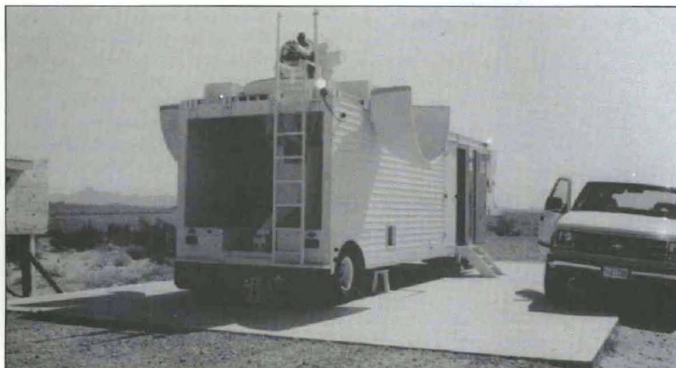
The mobile laser tracking system is a self contained unit capable of being transported anywhere.
