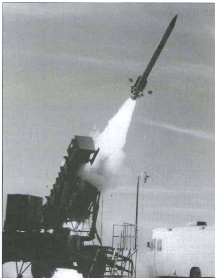
An ERINT missile is fired from White Sands Missile Range, NM, during developmental testing. The technology was developed in the early 1980s by the U.S. Army Space and Strategic Defense Command and has since been selected as the Patriot Advanced Capability-3 missile (PAC-3).
