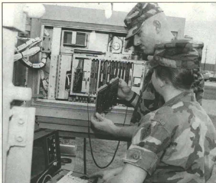
Figure 2. Soldiers testing Sentinel signal/data processor circuit card assembly.
