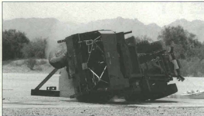
Shown above is the PLS truck as it rolls over on a specially engineered ramp.
