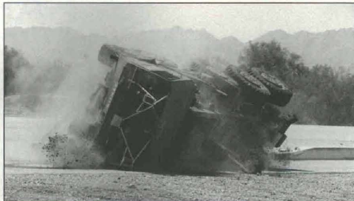
Shown above is the PLS truck as it rolls over on a specially engineered ramp.
