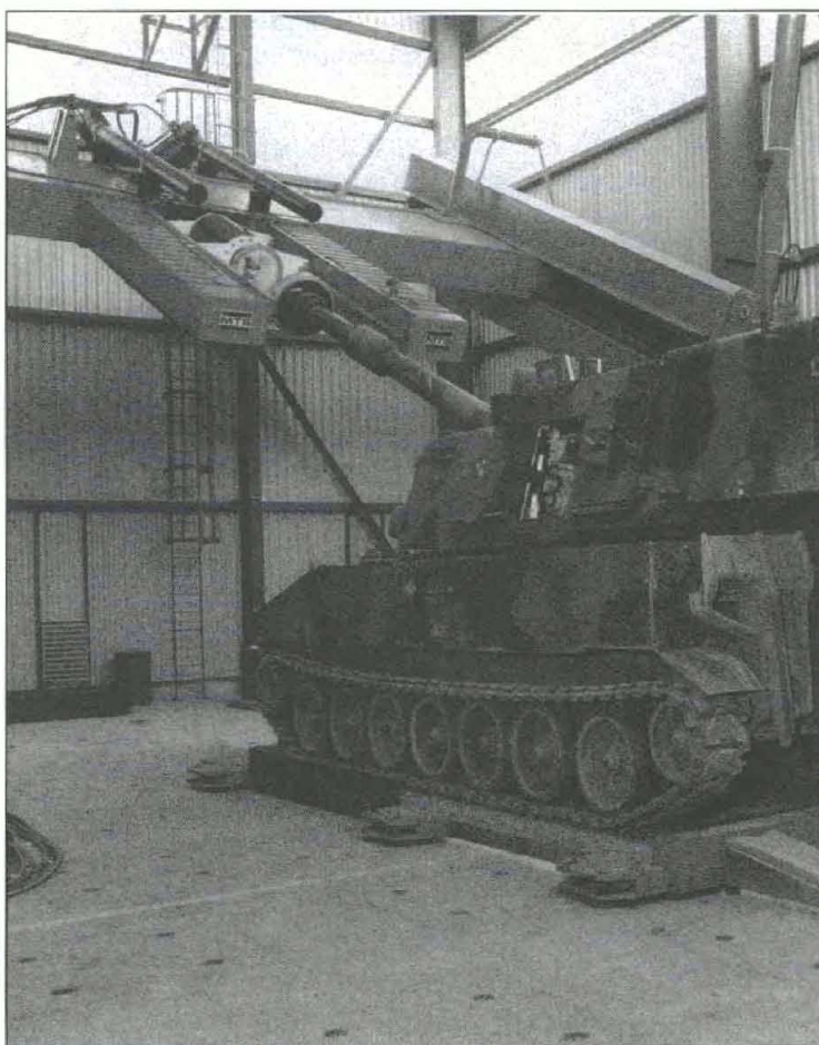
Figure 2. 155mm self-propelled Howitzer undergoing testing using Firing Impulse Simulator
