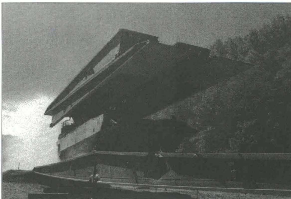
Figure 1. Wolverine Heavy Assault Bridge undergoing vulnerability testing
