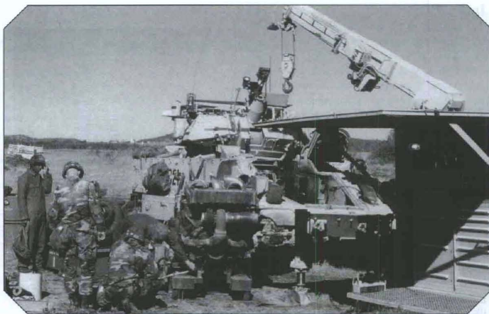
A forward repair system (FRS) crew working with a Bradley crew to repair and replace the Bradley's powerpack during the FRS IOTE with the 4th Infantry Division at Fort Hood in February 2000.
