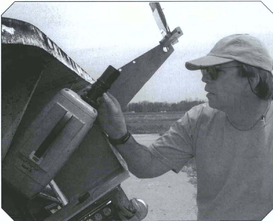
ATC employee Brett Patterson adjusts the digital camera to focus on a mirror above the protected armor plate. Camera is aimed at a mirror to "look down" the barrel of a tank gun to record the flight of a projectile as it appears to come directly at the camera.
