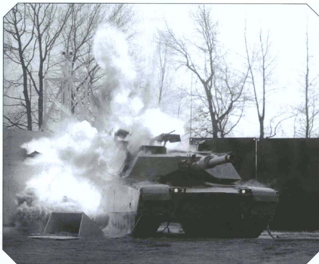
Specially designed blast housings and ruggedized cameras are used to document extreme testing at ATC.
