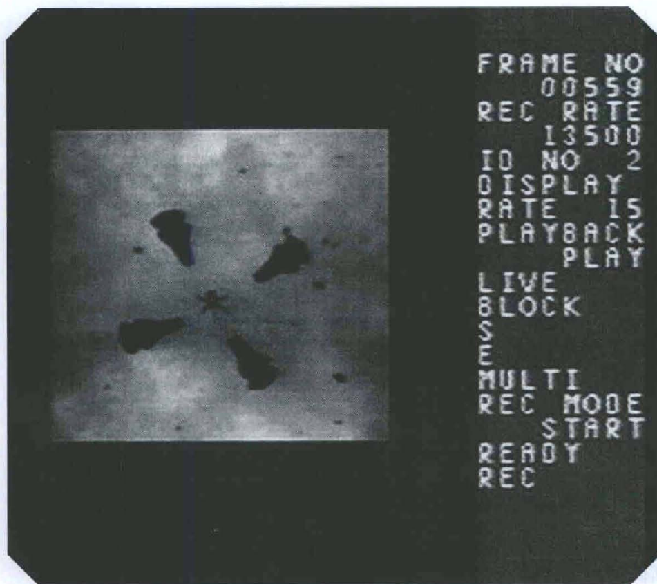
High-speed image looking down the barrel of a gun. Camera is positioned safely behind an armor plate under the line of fire with the lens aiming at a mirror to record the sabot separation as the projectile clears the fireball.
