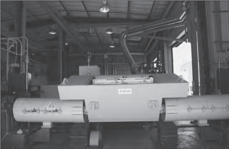
Termed "Hot Buck," the MGV Hybrid Propulsion Test Bed (shown here) at the U.S. Army Tank Automotive Research, Development and Engineering Center (TARDEC) Power and Energy Systems Integration Laboratory (SIL) in Santa Clara, CA, is a one-of-a-kind virtual FCS test bed platform for full-load testing. The Hybrid Propulsion Engine improves mobility, reduces fuel consumption and enables use of future weapon technologies. (Photos courtesy of BAE Systems.)
