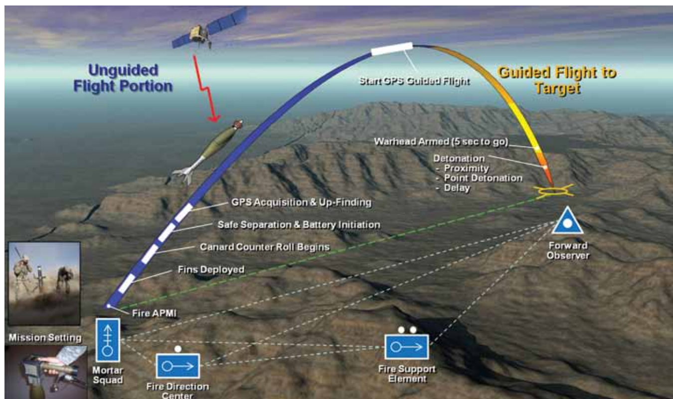
Accelerated Precision Mortar Initiative (120mm APMI) Operational Concept
