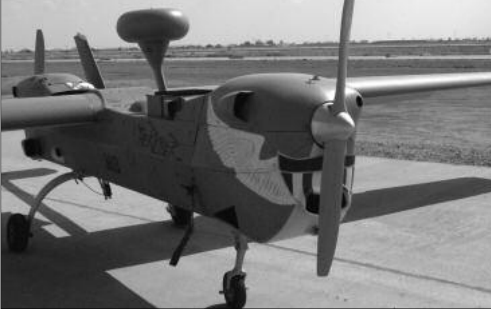
An Alpha Co., 15th Military Intelligence Battalion, Hunter UAS from Fort Hood, TX, awaits an operational deployment in Iraq. The Hunter UAS is being operationally integrated into the U.S. Army's divisional CAB structure to enhance RSTA assets in the fight against IED placement and discovery. (U.S. Army photo by Tarah Hollingsworth.)
