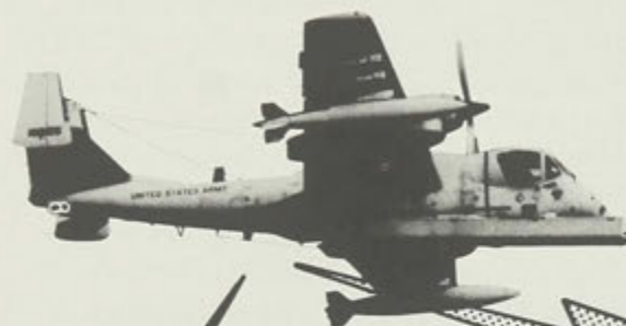
OV-1D MOHAWK AIRCRAFT W/ AN/APS-94F SIDE LOOKING RADAR (SLAR) AN/AKT-18B( ) AIRBORNE DATALINK (ADL)
