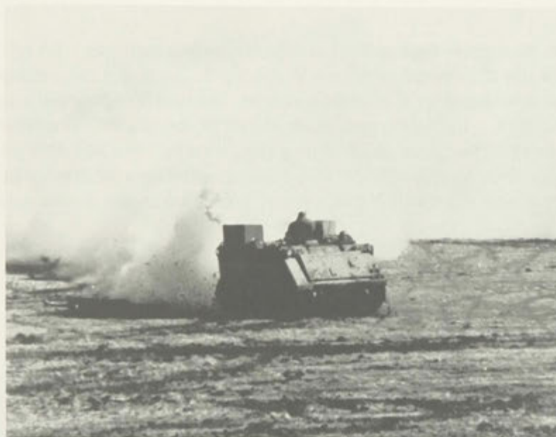
SMOKE GENERATOR SYSTEM MAKING A LARGE AREA SMOKE SCREEN
