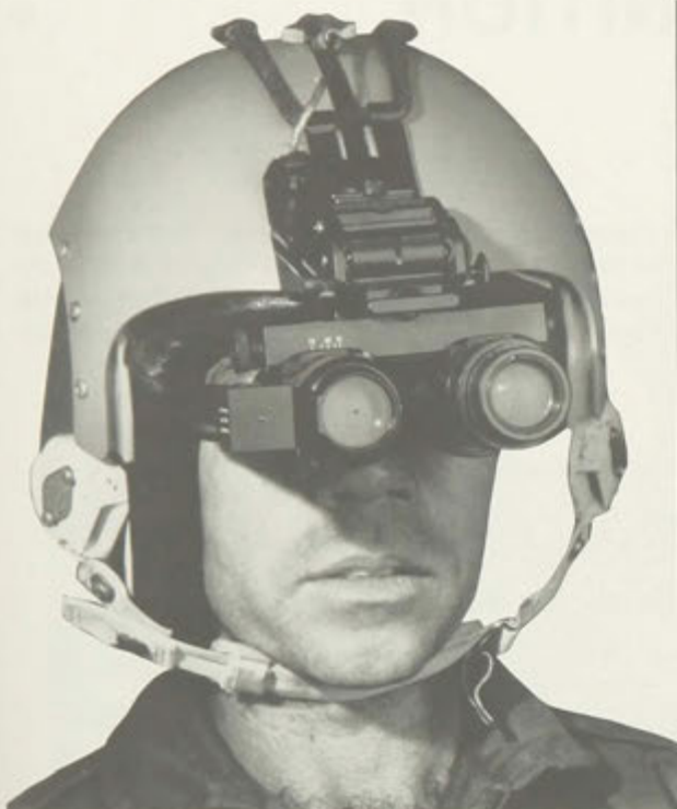
AVIATOR'S NIGHT VISION IMAGING SYSTEM WITH HEADS-UP DISPLAY
