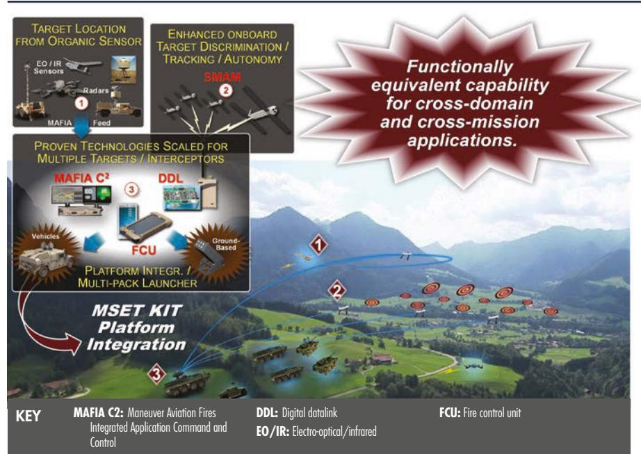
AMRDEC initiated a rapid prototyping effort for MSET in 2016 that involved modifying and integrating existing technologies to demonstrate concept feasibility. The goal was for a single operator to be able to fire and control six loitering precision missiles against four static targets and two moving targets, using an Android application to simultaneously control the surrogate missiles and then sequentially perform the terminal engagements.
